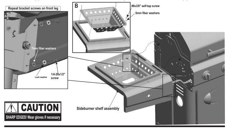
First, remove the two screws from the sideburner valve bracket. Align sideburner valve bracket behind sideburner shelf fascia with bezel on same level. Secure them altogether with two **#8-32x3/8"** screws. Press sideburner control knob onto valve stem.
